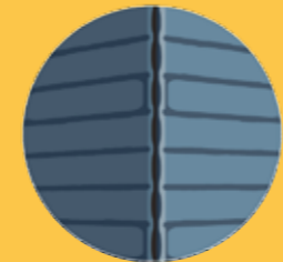
Corners - Raise /lower panels to align features. Mark position of corner, cut to form mitre. Fix panels leaving approx. 5mm gap, apply jointing compound and shape to suit
