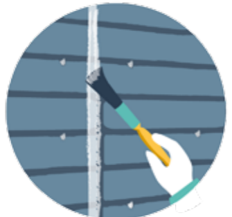
5 Introduce final texture to jointing compound with brush dipped in cleaner
