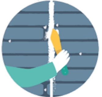
3 Roughly apply jointing compound to cover joints and fixing positions
