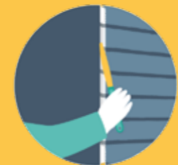
Finishing exposed edges - If panel end is exposed, use jointing compound to fill panel edge and shape as required
