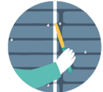
4 Shape the jointing compound to suit as it begins to go firm
