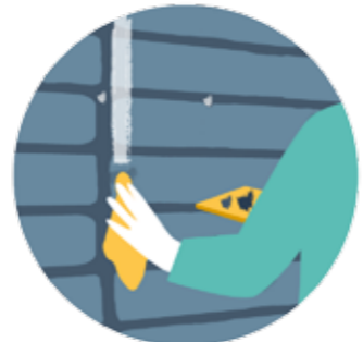
6 Leave for 24 hours, sparingly apply colour solutions, rag off and blend with surrounding area
