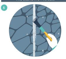
Introduce final texture to the jointing compound with a brush moistened with the cleaner.
