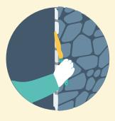
FINISHING EXPOSED EDGES - If panel end is exposed, use the jointing compound to fill panel edge and shape to create the stone end.
