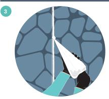
Use a grouting bag for the initial application of the jointing compound to cover joints and fixing locations.
