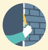
FINISHING EXPOSED EDGES - If panel end is exposed, use the jointing compound to fill panel edge and shape to create the brick end.
