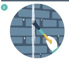
Introduce final texture to the jointing compound with a brush moistened with the cleaner.
