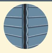
**CORNERS** - Raise or lower panels to align features. Mark position of corner and cut to form mitre.
