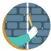
Raise or lower panels to align features, predrill and screw in place, packing out to suit
