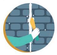
Leave for 24 hours. Apply colour solutions sparingly (avoiding bold strokes) to blend in with surrounding tones, and rag off before it dries
