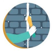
Leave for 24 hours. Apply colour solutions sparingly (avoiding bold strokes) to blend in with surrounding tones, and rag off before it dries
