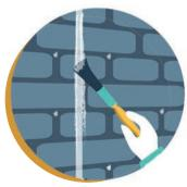
Roughly apply jointing compound (supplied) to cover joints and fixing positions
