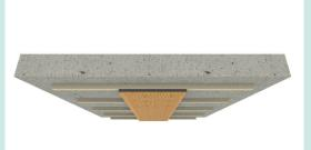
1 Lift panel to preinstalled ceiling substrate/rails.
