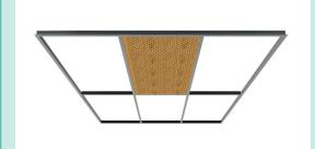
2 Swing the other edge up into the grid, shift and drop panel slightly to engage with the grid.
