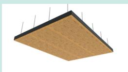
Repeat for remaining panels, cover edges with finishing strips.
