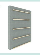
1. Fix the male parts to the wall substrate / rails, using the Click-Fix markers to position correctly.
