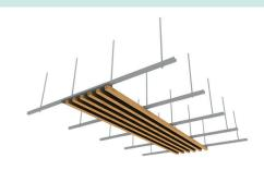
Lift Panel to pre-installed supports (Unistrut, Timber or similar - shown here suspended on rods).
