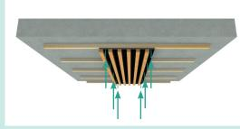
Screw through the panel backing and cross battens directly to the substrate, using discreet black screws in the black gap between the slats.
