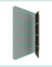
Install Hockey Sticks to wall substrate & Panel Rear in correct positions
