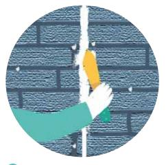
3 Roughly apply jointing compound to cover joints and fixing positions
