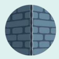
Corners - Raise /lower panels to align features. Mark position of corner, cut to form mitre. Fix panels leaving approx. 5mm gap, apply jointing compound and shape to suit
